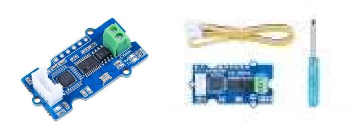
The I2C CAN Bus Module uses I2C for communication. Default I2C Address 0x25 and Max I2C Speed of 400k.
