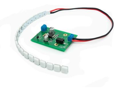
Dione Maxi consists of an array of MEMS speakers and the external amplifier to drive them. The speaker array, which is also referred to as the sound stripe, includes 20 USound Adap speakers connected in parallel. Due to its flexible structure and protective construction, the sound stripe is ideal for applications where audio is added on top of an existing design.
