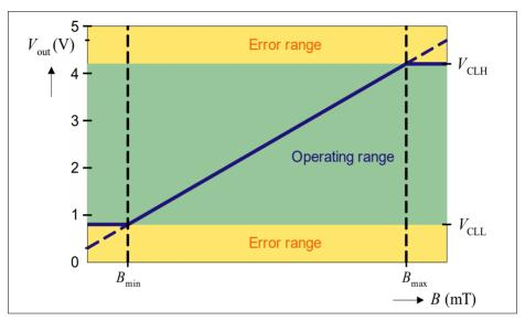
Figure 8 Clamping Example
