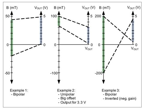
Figure 3 Examples of Operation
