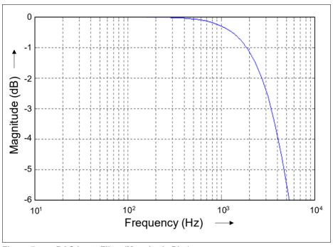
Figure 7 DAC Input Filter (Magnitude Plot)
