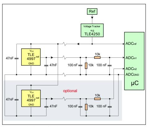
Figure 10 Application Circuit
