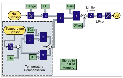
Figure 5 Signal Processing Flow
