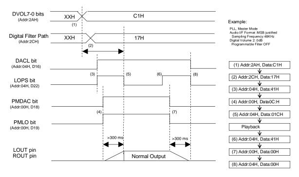
Figure 73. Stereo Lineout Sequence
