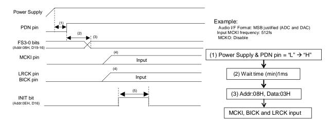
Figure 69. Clock Set Up Sequence (4)
