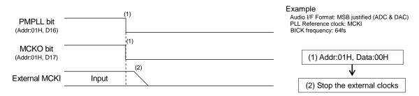
Figure 78. Clock Stopping Sequence (3)
