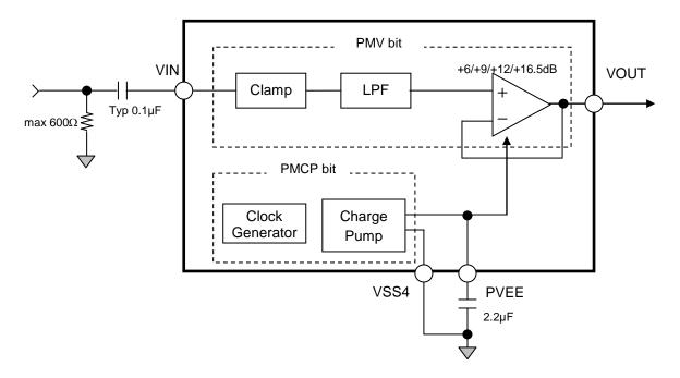
Figure 49. Video Block Diagram
