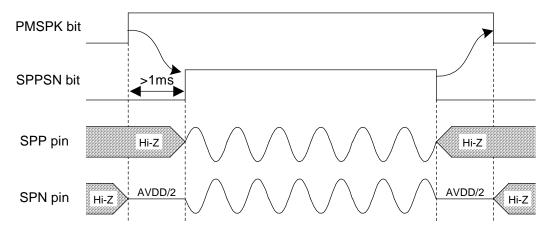
Figure 48. Power-up/Power-down Timing for Speaker-Amp
