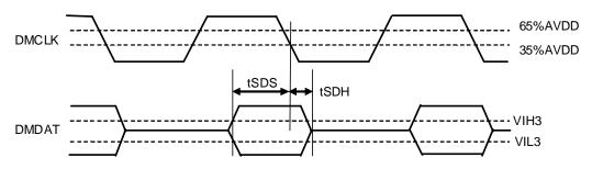
Figure 14. Audio Interface Timing (DCLKP bit = "1")
