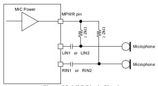
Figure 27. MIC Block Circuit
