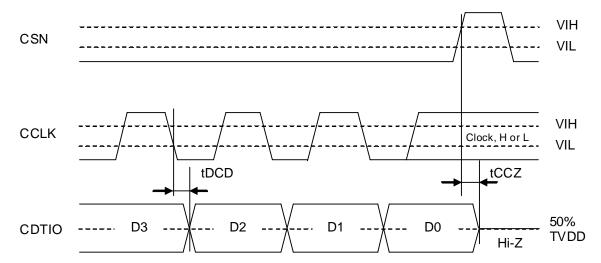
Figure 11. Read Data Output Timing
