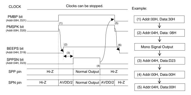
Figure 74. "MIN-Amp → Speaker-Amp" Output Sequence
