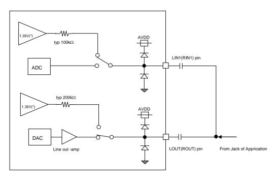
Figure 45. DAC→ LOUT/ROUT path: External Line Share (PMADC = LOPS bits = "0", EXTC bits = "1")
