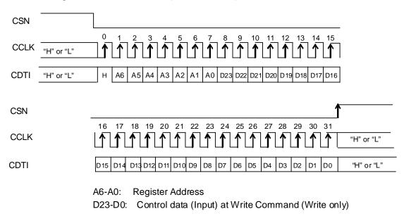
Figure 52. 3-wire Mode Control Interface Timing (COEW bit = "0")
