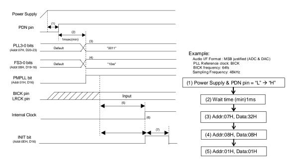
Figure 67. Clock Set Up Sequence (2)
