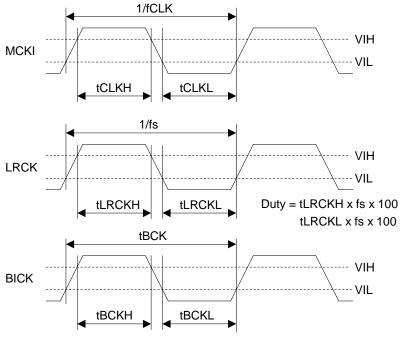
Figure 7. Clock Timing (EXT Slave mode)
