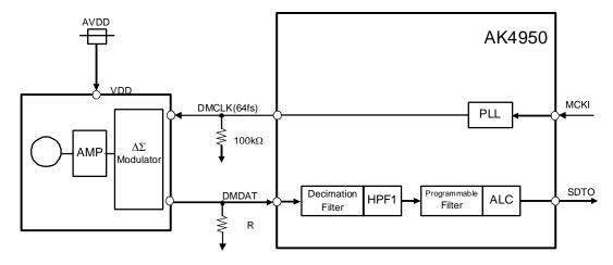
Figure 29. Connection Example of Mono Digital MIC
