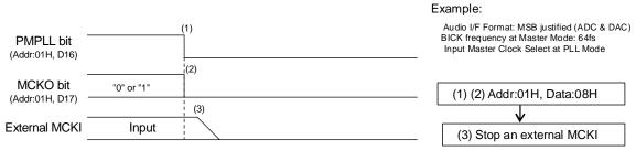
Figure 76. Clock Stopping Sequence (1)
