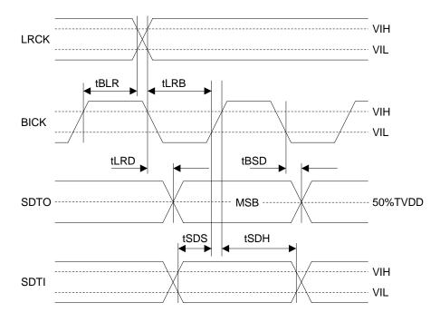
Figure 8. Audio Interface Timing (PLL/EXT Slave mode)
