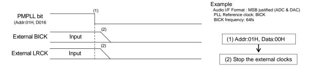
Figure 77. Clock Stopping Sequence (2)
