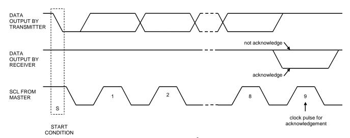
Figure 63. Acknowledge (I<sup>2</sup>C Bus)
