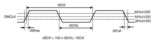
Figure 13. DMCLK Clock Timing
