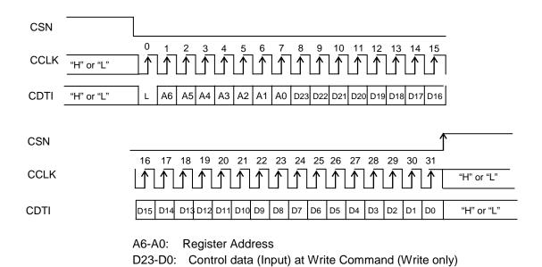
Figure 53. 3-wire Mode Control Interface Timing (COEW bit = "1")
