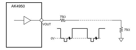
Figure 50. Video Signal Output
