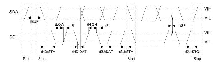
Figure 12. I<sup>2</sup>C Bus Mode Timing
