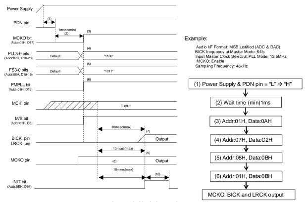
Figure 66. Clock Set Up Sequence (1)
