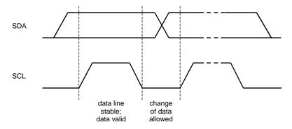
Figure 64. Bit Transfer (I<sup>2</sup>C Bus)
