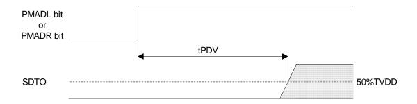
Figure 16. Power Down & Reset Timing 1
