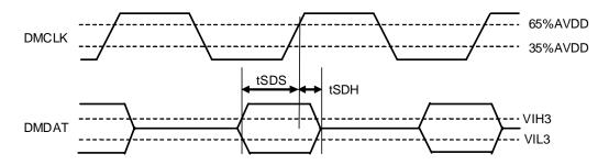
Figure 15. Audio Interface Timing (DCLKP bit = "0")
