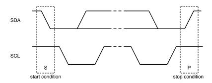
Figure 62. Start Condition and Stop Condition
