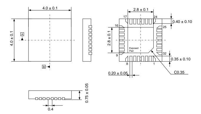
Note: The exposed pad on the bottom surface of the package must be connected to the ground.
