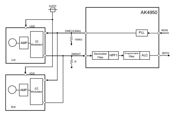
Figure 28. Connection Example of Stereo Digital MIC
