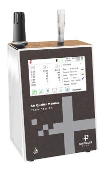
The Particles Plus® 7501-30 Remote Particle Counter measures 0.5 to 75.0 µm with a flow rate of 0.1 CFM (2.83 LPM). Easy to configure, this instrument displays up to 6 user-selectable size channels as well as temperature and relative humidity. View data and generate ISO 14644-1, EU GMP Annex 1 or FS 209E reports on screen or via printer, USB key, real time through its versatile output options or export to Particles Plus® Instrument Management Software.
