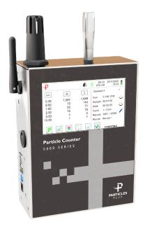
The Particles Plus® 5501-30 Remote Particle Counter measures 0.5 to 75.0 µm and are the most feature advanced remote particle counters available.
