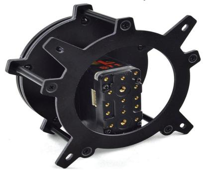
The main structure is made of four G10 composite plates and five aluminum standoffs. The four point mounting at the base is compatible with Lynxmotion's BR-KT base rotation kit, allowing it to be retrofitted on Lynxmotion robots. Lynxmotion servo sold separately.
