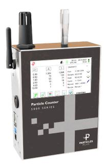
The Particles Plus® 5301P and 5501P Remote Particle Counters measure 0.3 or 0.5 to 25.0 µm and are the most feature advanced remote particle counters available. Integration is easy into a building automation and cleanroom management system via Ethernet, or (optional) Wireless 802.11 b/g, RS485 or RS232. Integrated web server displays instrument screen through any browser.
