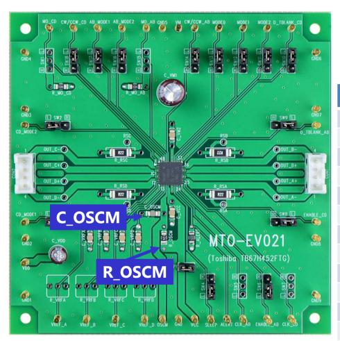
Set the chopping frequency by referring to the table shown below. The resistor of 120 k $\Omega$  is adopted to R\_OSCM and the capacitor of 270 pF is adopted to C\_OSCM in order to provide the frequency of 100 kHz at the time of shipment.
