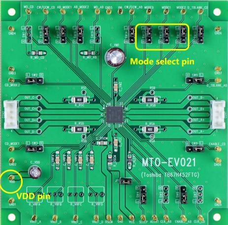
This evaluation board has a level select pin for setting the operation of the TB67H452FTG (shown in the photo below).
