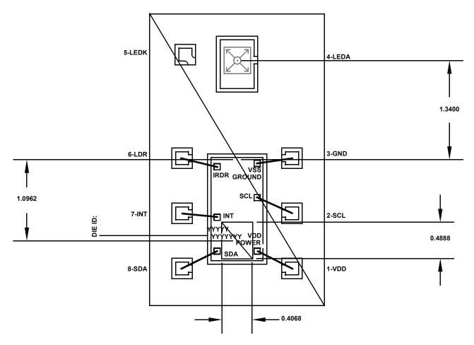
FIGURE 23. OPTICAL SENSOR LOCATION
