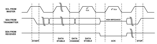
FIGURE 17. START, DATA STABLE, ACKNOWLEDGE, AND STOP CONDITION
