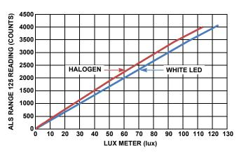
FIGURE 7. ALS TRANFER FUNCTION 2 LIGHT SOURCES (125 LUX RANGE)
