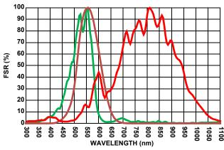
FIGURE 5. ISL29044 SENSITIVITY TO DIFFERENT WAVELENGTHS
