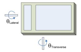
FIGURE 14. DEFINITION OF LATERAL AND TRANSVERSE AXES
