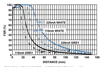
FIGURE 8. PROX COUNTS vs DISTANCE WITH 10cmx10cm REFLECTORS
