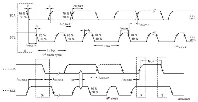
FIGURE 3. I<sup>2</sup>C TIMING DIAGRAM
