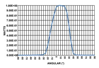
FIGURE 12. RADIATION EMISSION PATTERN IRLED TRANSVERSE
