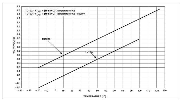
Figure 5. Output Voltage vs. Temperature
