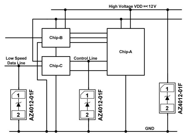
Fig. 2 ESD protection scheme for internal PCB circuits by using AZ4012-01F.
