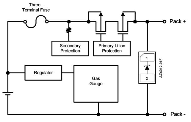
Fig. 1 ESD protection scheme for a typical Li-ion battery pack by using AZ4012-01F.
