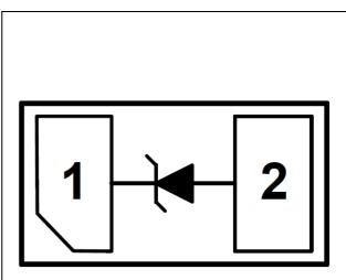
DFN1006P2X (Bottom View) (1.0mm x 0.6mm x 0.45mm)
