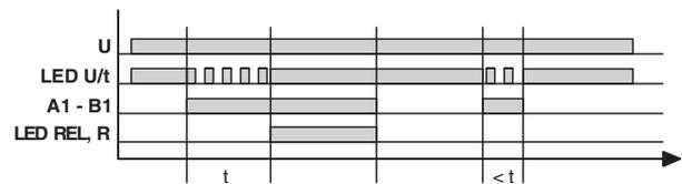
**Rs: With release delay and control contact**
