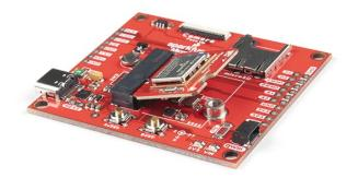
The Processor Board will stick up at an angle (at around 20°), as seen here:
