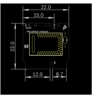
Each processor board follows the M.2 standard of '2222' or 22x22mm overall size.
