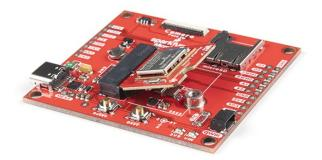
A MicroMod processor board is approximately 22x22mm and can insert into any MicroMod carrier board. A small screw holds the processor board in place. Whereas the original M.2 standard was designed for swapping out peripherals (user could change one solid state hard drive to a larger one) the MicroMod standard is designed for swapping out controllers (user can start with a powerful processor and then change to a low power controller to extend battery life).
