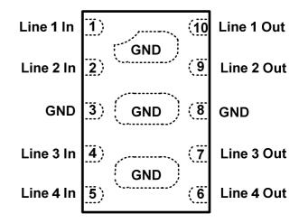
Fig. 1 Pin configuration of AZ3125-08F.
