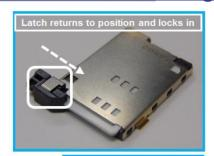
SIM Card is fully inserted
