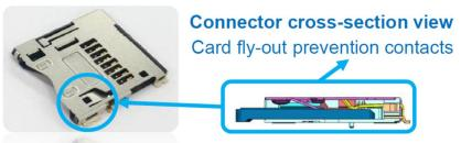
SIM cards' ejection speed are reduced by the stopper contacts to prevent unexpected flyout motion.
