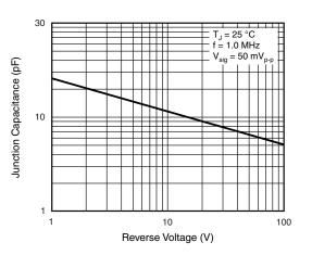
Fig. 5 - Typical Junction Capacitance
