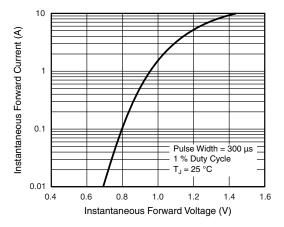
Fig. 3 - Typical Instantaneous Forward Characteristics
