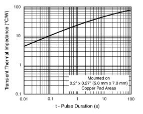
Fig. 6 - Typical Transient Thermal Impedance
