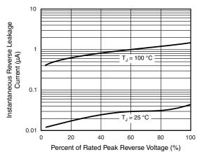
Fig. 4 - Typical Reverse Characteristics
