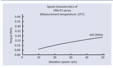
■ **Speed characteristics:** A rotary damper's torque varies according to the rotation speed. In general, as shown in the graph above, the torque increases as the rotation speed increases, and the torque decreases as the rotation speed decreases. In addition, please note that the starting torque slightly differs from the rated torque.
