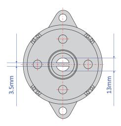
The FDT-63B-703 has a slotted groove which is excellent for usage with spiral springs
