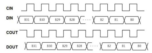
The serial command is transmitted with MSB first, DIN is latched at the rising edge of CIN clock. COUT and DOUT are re-generated for the next RGB LED. COUT is inverted from CIN. When 32 consecutive 0's are encountered, the next 1 is expected to start a 32-bit command, i.e., FLAG[2:0]=111. When FLAG[2:0]=111, then DIMMING, GREEN, BLUE and RED fields are latched respectively.
