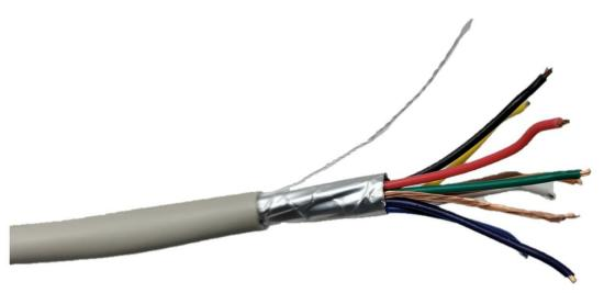
These 24AWG (American Wire Gauge) 9 bare copper conductor RS-232 multiconductor cables are used to create serial patch cables for a wide variety of applications, usually for computer peripherals.
