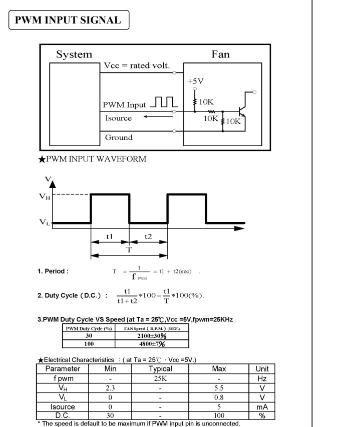
\* Min. start up duty cycle is 30%. Please don't apply 1 ~ 29% duty cycle to prevent unstable fan speed.
