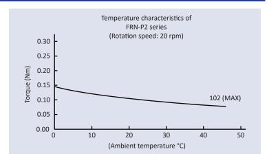
■ Temperature characteristics: A rotary damper's torque varies according to the ambient temperature. In addition, as shown in the graph above, the torque decreases as the ambient temperature increases, and the torque increases as the ambient temperature decreases. This is because the viscosity of the silicone oil inside the damper varies according to the temperature. When the temperature returns to normal, the torque will return to normal as well.
