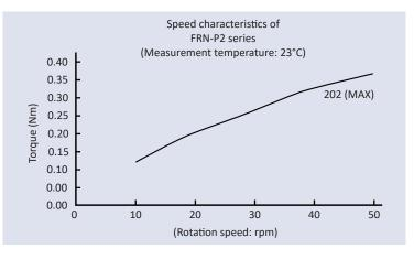
■ Speed characteristics: A rotary damper's torque varies according to the rotation speed. In general, as shown in the graph above, the torque increases as the rotation speed increases, and the torque decreases as the rotation speed decreases. In addition, please note that the starting torque slightly differs from the rated torque.
