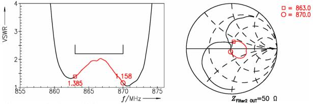
Figure 9: Reflection coefficient at Filter2 OUT port.
