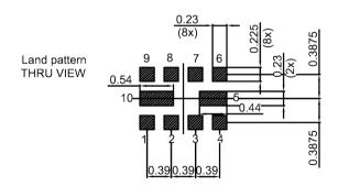
Landing pad tolerance -0.02 **Figure 2:** Drawing of package with package height A = 0.45 mm (max.). See Sec. Package information (p. 20).
