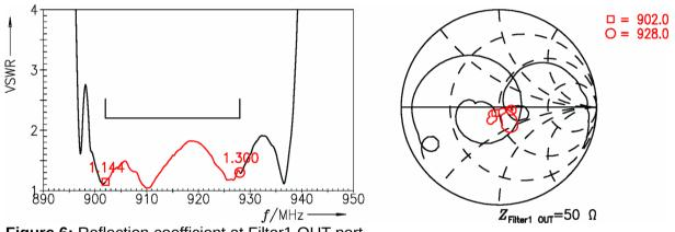
Figure 6: Reflection coefficient at Filter1 OUT port.
