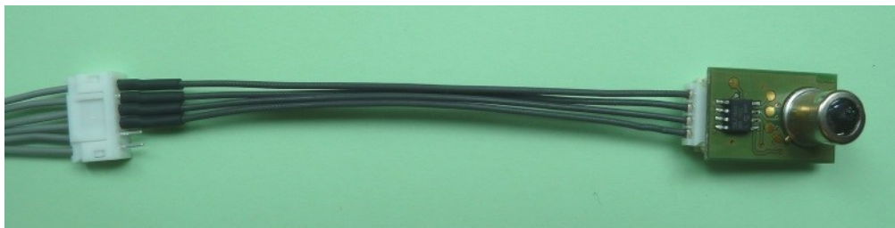
Figure 10: Connection of 4 pin boards through the JST adapter cable.
