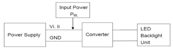
Note (2) At 20k Hz PWM control frequency , duty ratio range is restricted from 20% to 100%. Note (3) The lifetime of LED is estimated data and defined as the time when it continues to operate under the conditions at  $Ta = 25 \pm 2$  °C and Duty 100% until the brightness becomes  $\leq 50\%$  of its original value. Operating LED under high temperature environment will reduce life time and lead to color shift.
