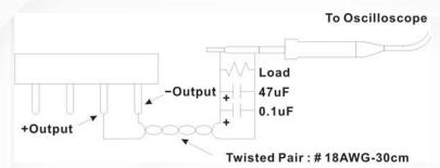
A 30cm twisted pair of no.18 AWG copper wire is connected to a 47uF and 0.1uF capacitor of proper polarity and voltage rating. The oscilloscope probe ground led should connect right to the ground ring of the probe and be as short as possible. The oscilloscope bandwidth should be at 20MHz and connected to AC ground.
