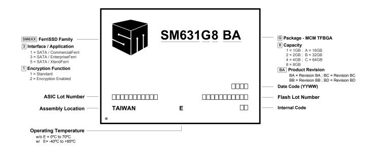
Figure 3: FerriSSD Single-Packaged SSD Top Marking – BD (Example)
