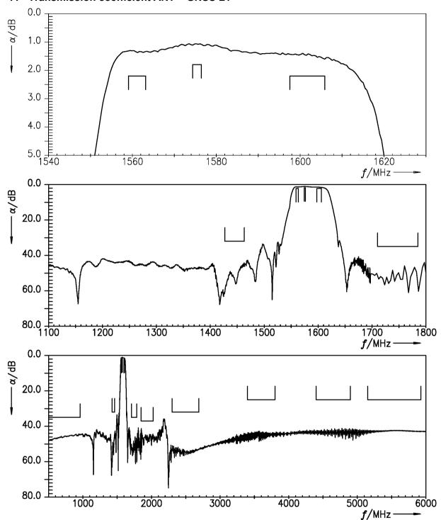
Figure 6: Attenuation ANT – GNSS L1.
