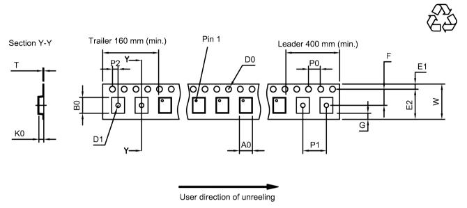
**Figure 9:** Drawing of tape (first-angle projection) for illustration only and not to scale. The valid tape dimensions are listed in Table 1.
