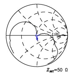
Figure 4: Reflection coefficient at ANT port.
