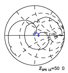
Figure 5: Reflection coefficient at GPS L5 port.
