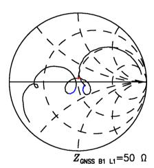
Figure 8: Reflection coefficient at GNSS L1 port.
