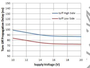
Figure 6. Turn-off Propagation Delay vs. Supply Voltage
