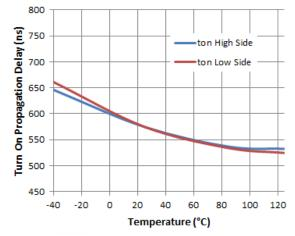
Figure 5. Turn-on Propagation Delay vs. Temperature
