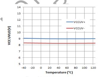
Figure 26. VCC UVLO vs. Temperature
