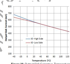
Figure 19. Output Sink Current vs. Temperature
