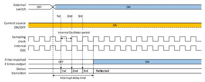
Time from Monitoring to End of Filtering:
