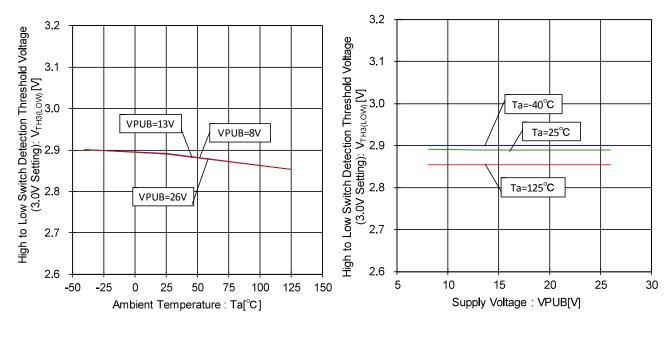
Figure 73. High to Low Switch Detection Threshold Voltage - Temperature Characteristic (3.0V Setting)
