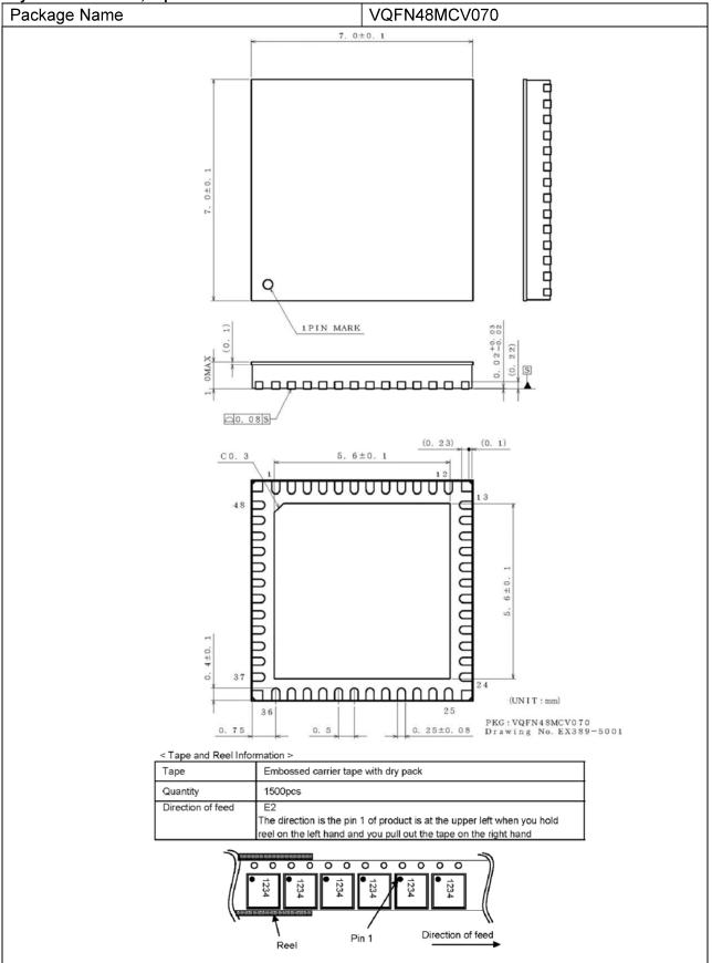
Figure 126. Physical Dimensions, Tape and Reel information
