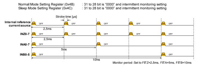
Figure 14. Intermittent Monitoring at the Same Time Example
