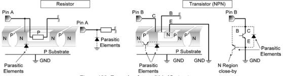
Figure 123. Example of monolithic IC structure
