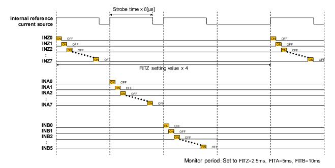
Figure 16. Sequential Monitoring of All Switches Terminals Example
