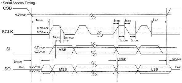
Figure 4. Serial Access Timing
