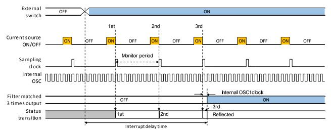
Time from Monitoring to End of Filtering:
