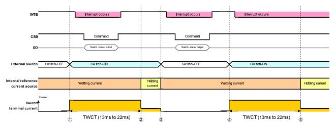
Figure 17. Wetting Current Timer (Continuous Operation)
