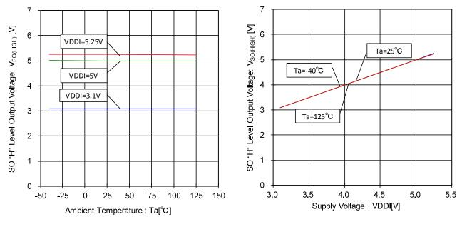
Figure 89. SO "H" Level Output Voltage- Temperature Characteristic ( $I_{SOURCE}$ =200 $\mu$ A)
