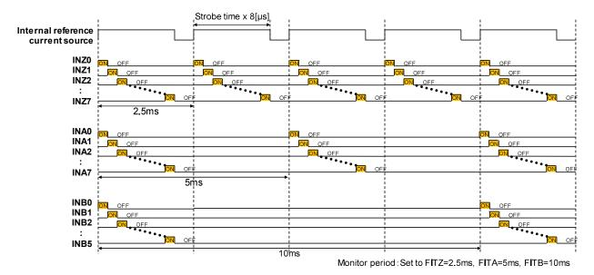
Figure 15. Sequential Monitoring by Power Supply System Example
