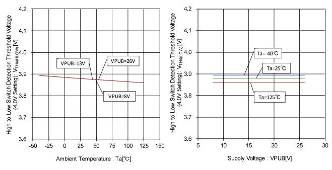
Figure 77. High to Low Switch Detection Threshold Voltage - Temperature Characteristic (4.0V Setting)
