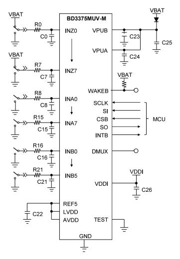
Figure 121. Example of Application Circuit and its External Components
