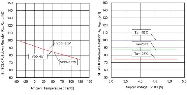
Figure 85. SI, SCLK Pull-down Resistor- Temperature Characteristic
