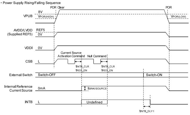
Figure 5. Power Supply Rising/Falling Sequence
