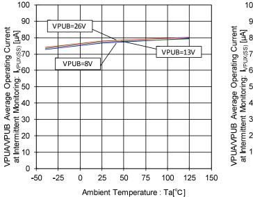
Figure 25. VPUA/VPUB Average Operating Current at Intermittent Monitoring - Temperature Characteristic (Monitoring Period: 50ms, Strobe Time: 125µs, Source/Sink Current Setting: 1mA)
