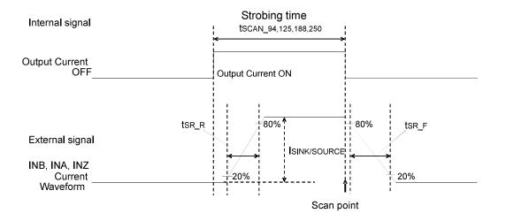
Figure 6. Intermittent Monitoring Enabled (FSQ=0, FSQZ/A/B=0, CMB/A/Z=1), Source/Sink Current Rise and Fall Time
