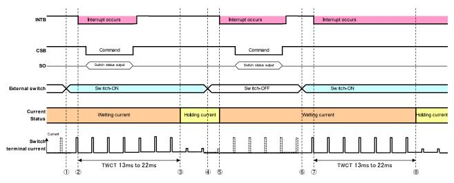
Figure 18. Wetting Current Timer (Intermittent Monitoring)
