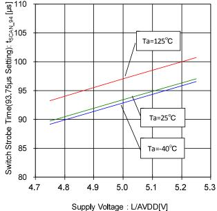
Figure 109. Switch Strobe Time- Temperature Characteristic (93.75µs Setting)
