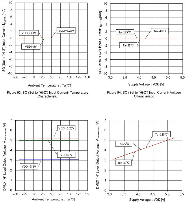
Figure 95. DMUX "H" Level Output Voltage-Temperature Characteristic (I<sub>SOURCE</sub>=200µA)
