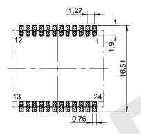
no vias or traces underneath the component Scale - 2:1
