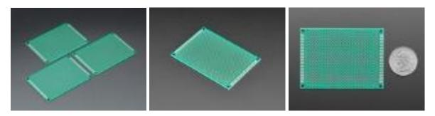
Here's a handy 3-pack of 5cm x 7cm Proto-board PCBs in green. Both sides have a green silkscreen with some row/column markings. Note that these *don't* have any traces between the PCB holes, <u>you would normally bend over a thru-hole lead to create connections</u>. They're also good for just plain mechanical work because they are made of strong FR4.
