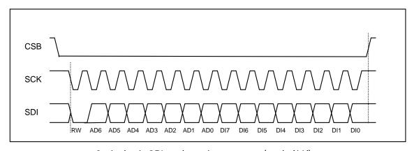
3-wire basic SPI read or write sequence (mode '11')
