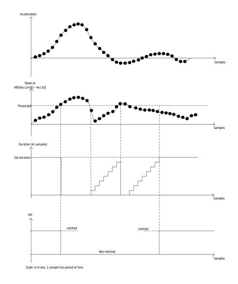
Register FEATURES\_IN.no\_motion.settings\_2.duration defines the number of consecutive data points for which the slope of enabled axis must be smaller than the threshold for an interrupt to be asserted.
