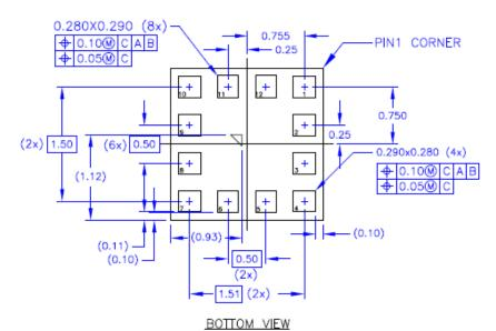
Note that the pin 5, 6, 11, 12 are in same direction (0.280\*0.290, 4x), while pin 1, 2, 3, 4, 7, 8, 9, 10 are in same direction (0.290\*0.280, 8x).
