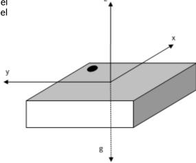
The following table lists all corresponding output signals on X, Y, and Z while the sensor is at rest or at uniform motion in a gravity field under assumption of a  $\pm 4g$  range setting, a 16 bit resolution, and a top down gravity vector as shown above.
