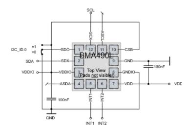
It is recommended to use 100nF decoupling capacitors at pin 3 (VDDIO) and pin 7 (VDD). SDA and SCL should be connected to  $V_{\text{DDIO}}$  externally via pull-up resistors so that they are pulled high when the bus is free.
