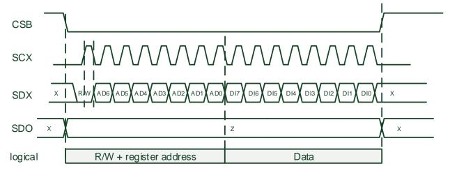
4-wire basic SPI write sequence (mode '00')
