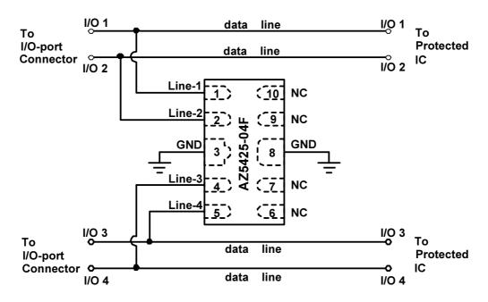
Fig. 1 Data lines connection of AZ5425-04F.
