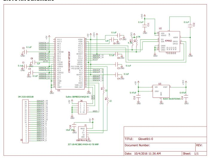
The heart of the USB kit is the Cypress PSoC CY8C3246PVI-147. The Cypress PSoC is a great part to use with Flexpoint Bend Sensors since they have an integrated current DAC. This allows the Bend Sensor® to be interfaced with the ADC directly without the need of any external components like voltage divider resistors or op-amps.
