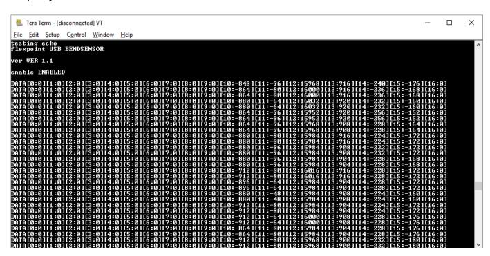
The USB Glove kit will echo any characters sent to make it easy to view in the terminal. The Glove kit responds to the following commands. The commands are lowercase and the responses are UPPERCASE.
