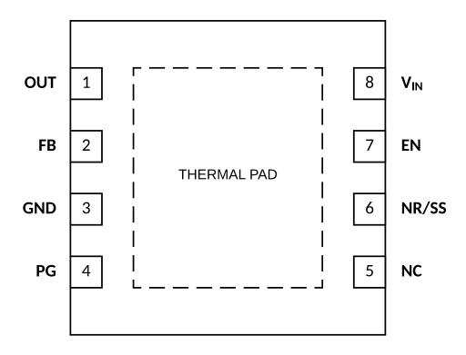
Figure 2 Au8011A Pin Configuration
