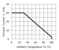
Fig. 3 FORWARD CURRENT VS. DERATING CURVE
