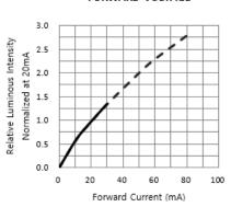
Fig. 4 RELATIVE LUMIOUS INTENSITY VS. FORWARD CURRENT
