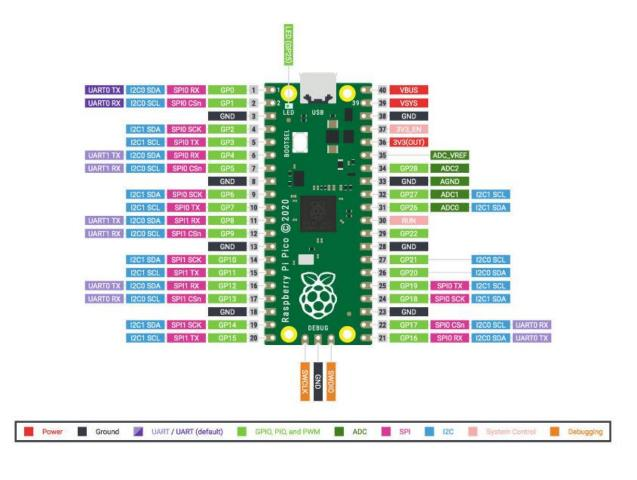
The Raspberry Pi Pico board, a new low cost, high-performance microcontroller. The board features a powerful new, Raspberry Pi designed ARM-based dual-core chip-- the RP2040. The pico also features 64KB of internal RAM and support for up to 16MB of off-chip Flash. A wide range of flexible I/O options includes I2C, SPI, and Programmable I/O (PIO). These support endless possible applications for this small and affordable board.
