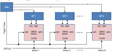
Figure 20. Trigger Mode Block Diagram
