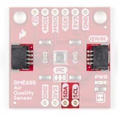
If you would prefer to communicate with your BME680 via SPI, we have broken those pins out as well to standard 0.1"-spade header pins. Communicating over SPI requires more connections than  $I^2C$  but is more versatile and can be faster. It is particularly helpful if you need to use more than two BME680's in your circuit or if you have other devices using the same  $I^2C$  addresses.
