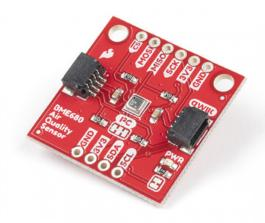
SparkFun Environmental Sensor Breakout - BME680 (Qwiic)
