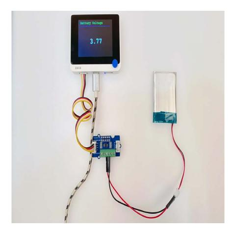
For communication, the module uses I2C communication with four optional I2C addresses, allowing for multi-chip cascading for more complex scenarios. With the Grove connector, you can connect Grove - ADS1115 with your Raspberry Pi and Arduino easily.
