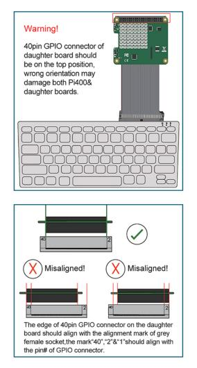
3.Please double check the orientation of daughter board and position of pin#1,2 & 40 base on the below chart before power on Pi400.
