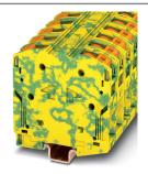
Ground modular terminal block, number of connections: 2, number of positions: 1, connection method: Power-Turn connection, 1 level, Rated cross section: 95 mm<sup>2</sup>, cross section: 25 mm<sup>2</sup> - 95 mm<sup>2</sup>, mounting type: 2.3 mm copper DIN rail, color: green-yellow
