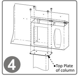
Attach the RS005-0233 Respiratory Hygiene Station to the column using (4x) screws included with stand. Tighten.
