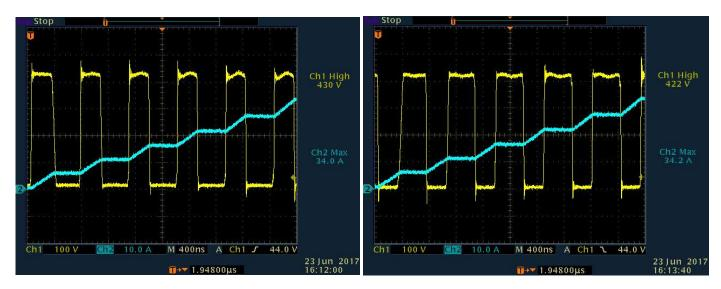
Fig 5. Hard-switched waveforms of a pair of GaN FET switches when setting a) high side as master and b) low side as master
