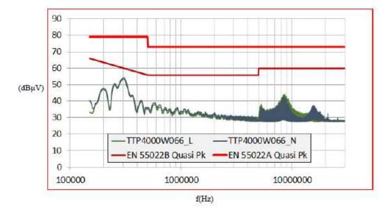
Fig 17. Conducted emissions @ 115V, 1150W
