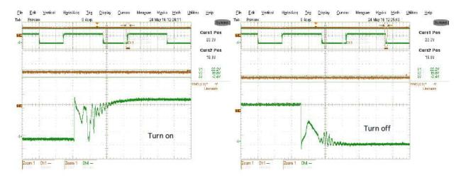
Fig 12 waveforms of Vgs of Q2 at iL = 23A. CH1: input current lin (10A/div); CH4: (a) Vgs of Q2 (5V/div)
