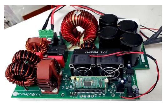
Figure 1. TDTTP4000W066B\_0v1 4kW totem-pole PFC evaluation board
