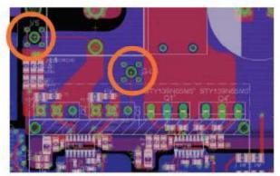
By removing the jumpers and using a short wire to clamp the current probe, the PFC inductor can also be measured.
