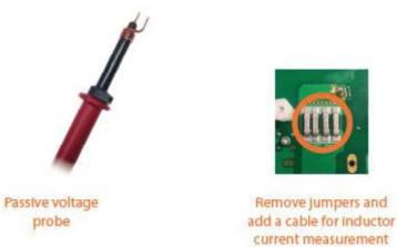
Fig 15. Vgs and Vds of Iow side GaN FET measurement socket tips, and PFC inductor current measuring position.
