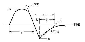
Figure 14. Diode Reverse Recovery Waveform
