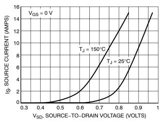
Figure 10. Diode Forward Voltage versus Current
