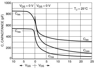
GATE-TO-SOURCE OR DRAIN-TO-SOURCE VOLTAGE (VOLTS)
