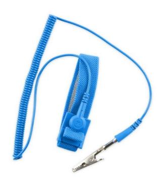
"Rapid static dissipation by a wrist strap ground is required to prevent voltage spikes. Simple movements such as lifting one foot off the floor or raising one arm from a conductive table mat may change body capacitance by as much as 10% to 30%. Uncontrolled, the capacitively created voltage may reach several hundred volts or more."
