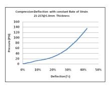
21-217Gap Pad 1.0mm thick; 1 inch^2 test sample; Rate of strain = 1.0 mm/min
