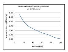
21-217 Gap Pad 1.0mm thick; 1 inch^2 test sample; Pressure step = 10psi
